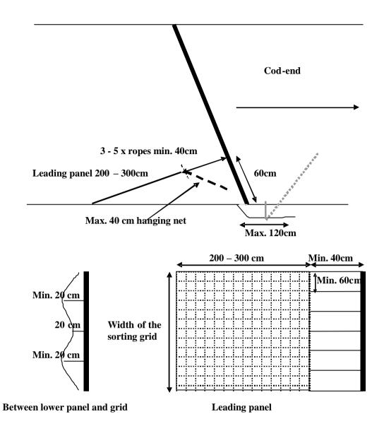
Illustration of the rigging and installation of a sorting grid in the trawl, with the latest modifications adding a leading panels in front of the grid and insertion of ropes to stabilise the escape opening.
